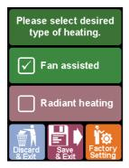
**Heating mode:** If a fan assisted heating system such as fan coil has been combined with radiant heating such as underfloor heating, you may select either of these methods or both of them for heating.
