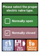
**Valve type:** Choose the type of actuator on the electromagnetic valves, if they are present. The available options are normally closed or normally open.
