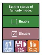
**♦ Fan only:** Enabling this option appends the "Fan only" mode to the operation modes of your thermostat on the main screen, as described on page 9. During this mode the air conditioner acts as a blower without heating or cooling the air.
