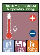
**6 Temperature swing:** Allowable room temperature fluctuation from the set point, when the thermostat is in operational mode. Touch "+" or "-" to set the temperature swing between 0.5°C and 1.5°C in 0.1°C steps.
