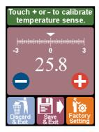
**Galibration:** Actual room temperature differs from point to point. Sensed temperature is precisely calibrated in the factory. To match the sensing with some specific point in the room, re-calibrate the thermostat by touching the "+" or "-" icon.
