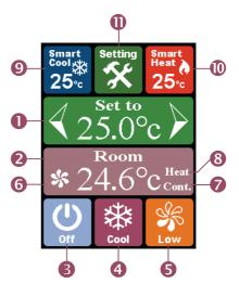
**NOTE** By Selecting the fan only mode  $\approx$ , the air conditioner blows air continuously without heating or cooling. To stop the blowing, switch the device to standby mode.
