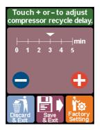
**D**Recycle delay: Successive restarts can damage the electro motor of a compressor owing to overload. A restart delay, about 3 minutes, is necessary to equalize the pressure. Touch "-" or "+" to set the compressor restart delay in minutes.
