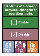
**Heat/Cool changeover:** This appends "Heat/Cool changeover" to operation mode. When selected, thermostat switches between heating or cooling whenever necessary. Not all air conditioners are capable of operating in this mode. Refer to page 9.
