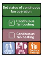
**3** Continuous fan status: Enabling this option for heating or cooling causes the fan never to switch off during Cooling or Heating mode, if available; instead it merely blows the air when the cooling or heating is no longer necessary.
