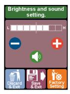
**4** Beep and Brightness: Touch '-' to dim down or '+' to brighten up the screen light. Also, you may touch the speaker sign to mute or unmute the touch beep. This has no effect on the confirmation beep sound for the remote controller.
