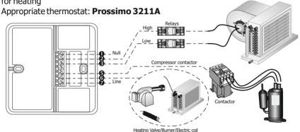
Terminal Input/ **Electrical** Description number Output characteristics Null 1 Input AC 220V / 24V 50Hz Fan high Output AC 220V / 24V 50Hz 3 Fan low Output AC 220V / 24V 50Hz 4 Do not connect 5 To compressor contactor Output AC 220V / 24V 50Hz To valve/electric coil relay/gas burner controller 6 Output AC 220V / 24V 50Hz 7 Line Input AC 220V / 24V 50Hz
