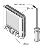
③ Release the back wall mounting plate. There are four latches, as illustrated in the figure, two at the top and two at the bottom of the thermostat. Use a screwdriver with a tip between 3 and 5 mm to gently release them. After releasing each of the latches, pull the respective device corner a little to keep the latch from snapping in again. Pull the device straight out from the back mounting plate after releasing all four latches.
