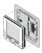
Mounting the unit: Hold the thermostat face parallel to the wall surface. Do not incline the thermostat face. Match the needles on the back of the thermostat with the holes on the terminals of the mounting plate. push the thermostat gently over the needles until the latches snap closed.
