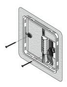
④ Position the mounting plate on the wall. Use a pencil to mark the mounting holes. Remove the plate from the wall and drill 3/16" holes in the wall. Tap anchors into the drilled holes. Reposition the plate and loosely insert two mounting screws in the holes. Level the plate for appearance. Tighten the mounting screws.
