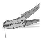
② Use a crimping tool to secure the wire ferrules supplied with the device on the wires to prepare them to be screwed into the terminals. The best wire size is AWG16 (1.5 mm diameter), but wires up to AWG12 (2.5 mm diameter) can also be used in the thermostat terminals.
