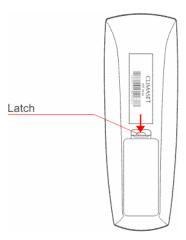
The cover releases. Lift off the cover to reveal the inner battery compartment.
